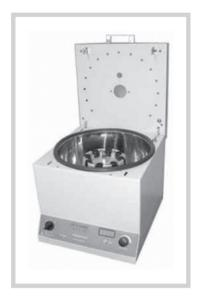
**FIG. 1.13:** Swing out head centrifuge (*Courtesy:* Yorco Sales Pvt. Ltd)
