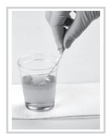
FIG. 5.12: Dip the reagent strip
