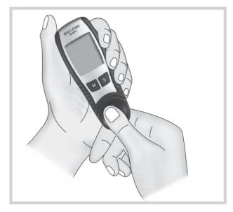
FIG. 17.9: Maintenance—opening the cover
