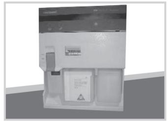
FIG. 21.5: Bayer 614 electrolyte analyzer
