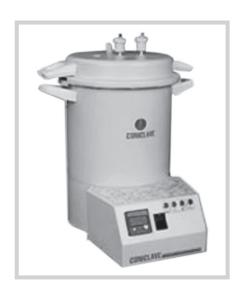
**FIG. 2.1C:** Precision autoclave (*Courtesy:* Yorco Sales Pvt. Ltd.)
