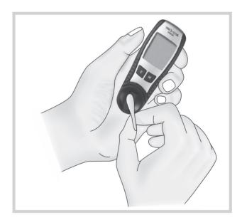
FIG. 17.10: Maintenance—cleaning the optics
