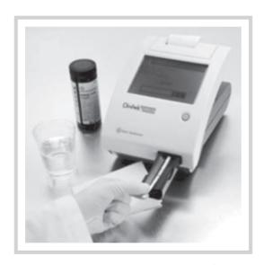
FIG. 5.13: Place reagent strip on the instrument feed table
