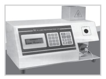
FIG. 21.2: Flame photometer
