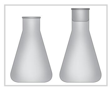
FIG. 1.17: Conical flasks
