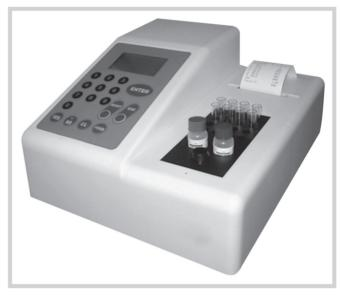
FIG. 23.17: Quantimate turbidimetry analyzer
