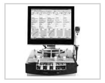
function testing is utilized in the analysis of inherited and acquired platelet function disorders that may cause a transient or permanent bleeding tendency. The Multiplate analyzer can detect platelet dysfunction and thus aid in the therapeutic management of such patients.
