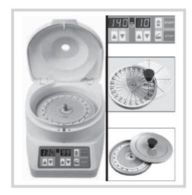
**FIG. 1.16:** Microhematocrit centrifuge and its parts (*Courtesy:* Yorco Sales Pvt. Ltd)
