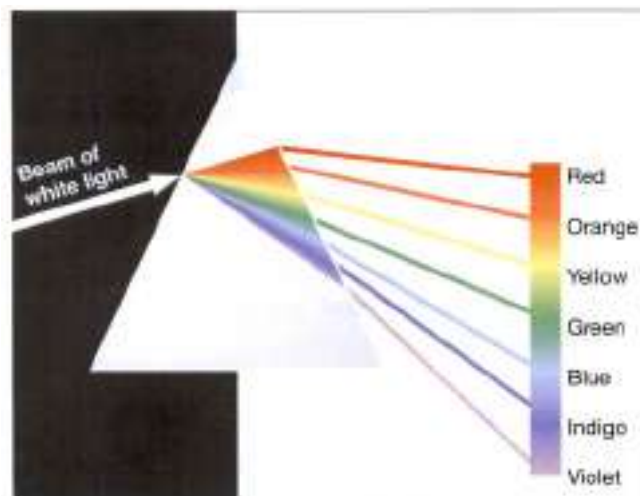
Figure 8.14 Refraction of white light broken into the colours of the visible spectrum when passed through a prism
