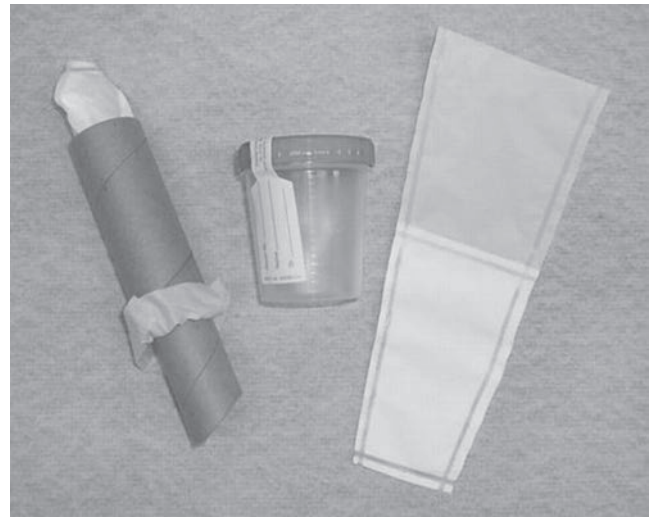
FIGURE 72-3 An X-Cell 200 HEPA vacuum sample kit with (left to right) disposable nozzle assembly, sterile sample container, and filter sock (Midwest Filtration Co., Cincinnati, OH).
