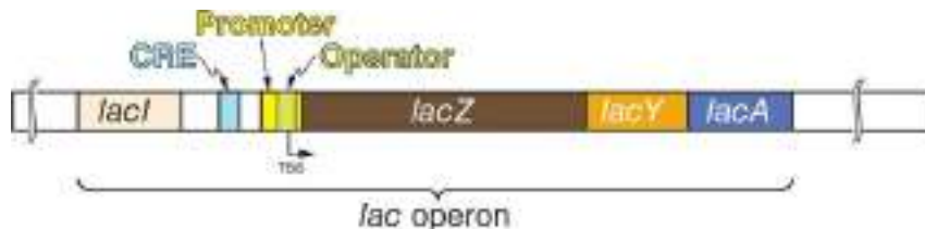
FIGURE 38–2 The positional relationships of the protein coding and regulatory elements of the ~6kbp lac operon. lacZ encodes \beta -galactosidase, lacY encodes a permease, and lacA encodes a thiogalactoside transacetylase. lacI encodes the lac operon repressor protein. Also shown is the transcription start site for lac operon transcription (TSS). Note that the binding site for the LacI protein (ie, lac repressor)—the lac operator (Operator) overlaps the lac promoter. Immediately upstream of the lac operon promoter is the binding site (CRE) for the cAMP-binding protein, CAP, the positive regulator of lac operon transcription. See Figure 38–3 for more detail.
