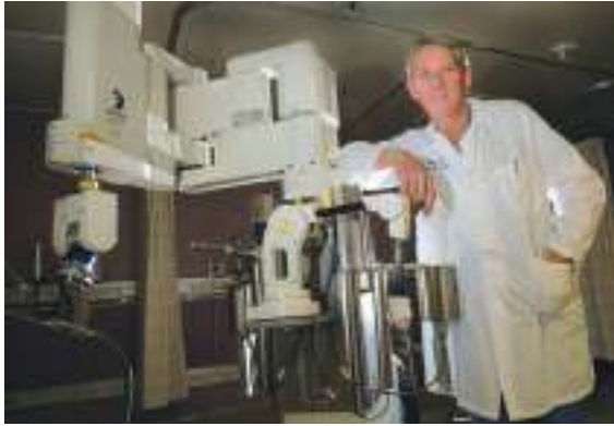
(c) Physician with the ROBODOC machine used to perform hip joint replacement surgery.
